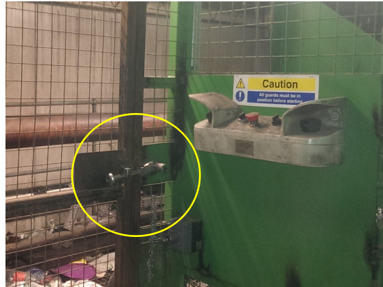
Bottle Piercer Isolation in Place
