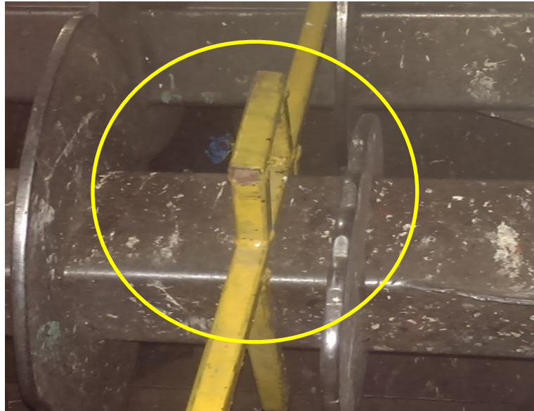
Correct Fit – Firmly down Both Sides of the Shaft ✓
