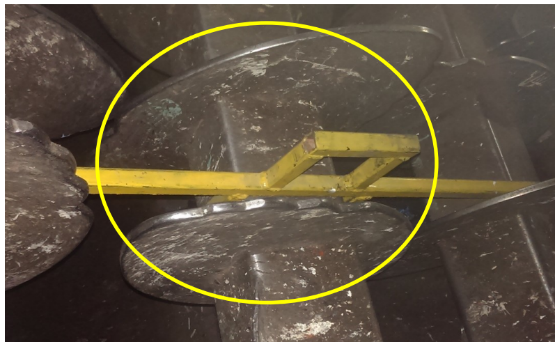
Correct Fit – Firmly down Both Sides of the Shaft ✓
