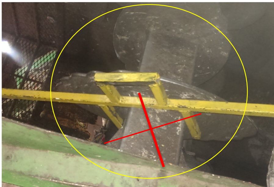
Incorrect Fit – NOT Placed Firmly around the Shaft X
